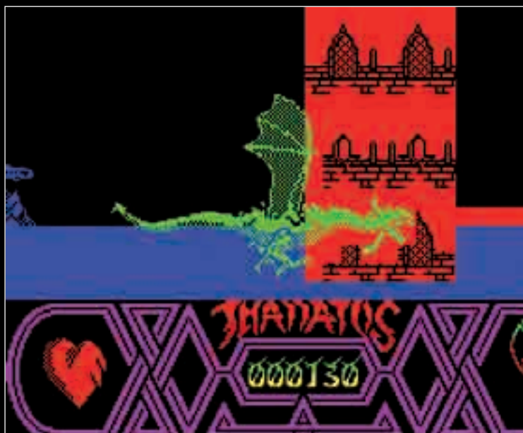
» As Thanatos flies past the castle wall, note how the background colour of the sprite's character squares switch to try to counter the Spectrum's nasty colour clash ailment.
